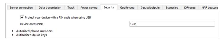
Protect your device with a PIN code when using USB – if there is a checkmark - when you start the "Configurator" program, when you try to connect to the device, you will be asked for the PIN code specified
